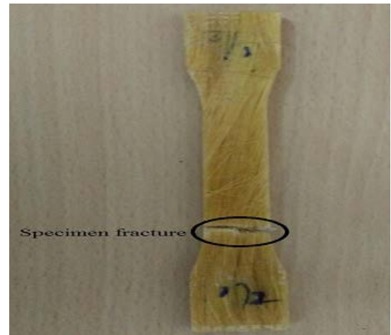
Figure 11: Tensile Test Specimen after Fracture
