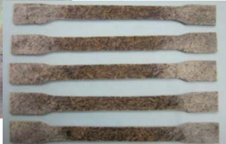
Figure 6: Tensile Test Specimens
