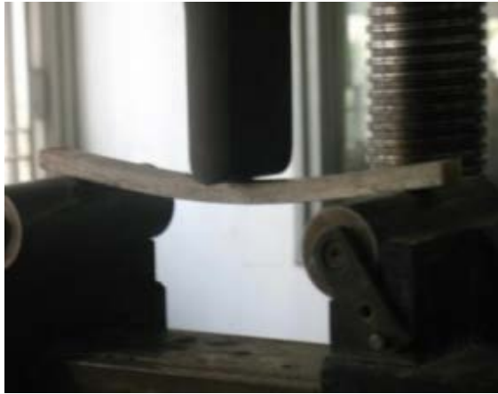
Figure 8: Flexural Test Arrangement
